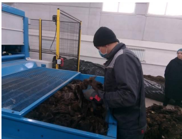
Fig. 15. Sheep wool being fed into the Cormatex deburring machine to remove organic and mechanical dross- an operation generating plenty of dust
