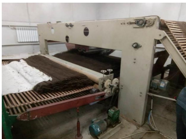
Fig. 16. Prefinished multi-layered wool felt after subsequent stages of treatment (combing, needle punching...)
